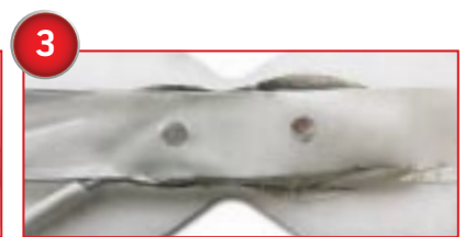
When the components are not removed from the original tape, it makes it difficult to align the components with the opening in the outer tape. This results in partially occluded components, compromising performance of the sensor.
