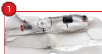
Internal tape layer is not removed from the components.
