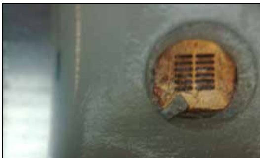
Figure 10. Embedded particle embedded in detector of third-party reprocessed sensor
