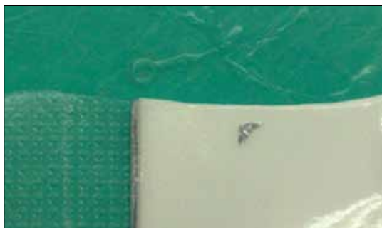
Figure 11. Embedded particle in adhesive of third party reprocessed sensor
