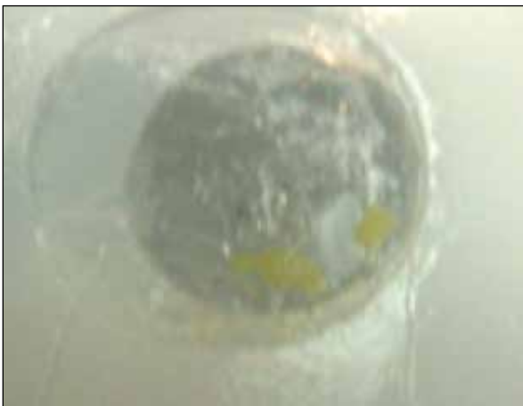
Figure 3. Yellow stain covering detector of third-party reprocessed sensor
