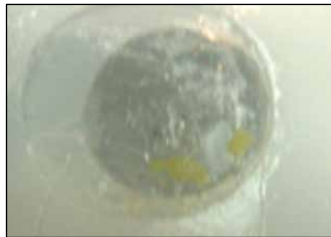
Yellow stain covering detector of third-party reprocessed sensor
