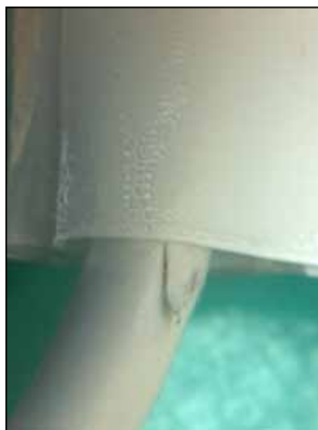
Figure 13. Chipped sensor cable on third-party reprocessed sensor
