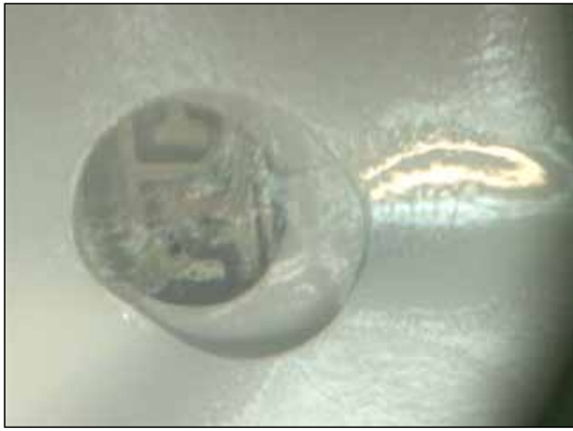
Figure 4. Third-party reprocessed sensor emitter obscured by glue and adhesive placement
