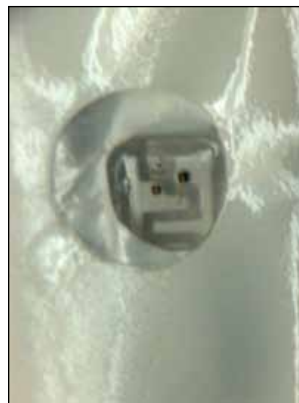
Figure 9. Transparent film over emitter on third-party reprocessed sensor missing
